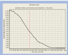
The X axis shows the wall cost, the Y axis the façade length above target values [m]. The façade length considers individual floors. The red line indicates the chosen wall configuration for the graphics panel which can be saved for further noise map calculations.
